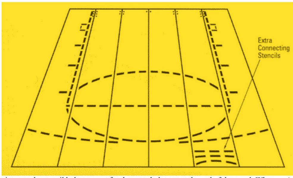
Roll the paint over the stencil holes, except for the extra holes out at the end of the panel. When you've finished painting, pull up the stencil: no need to wait.
