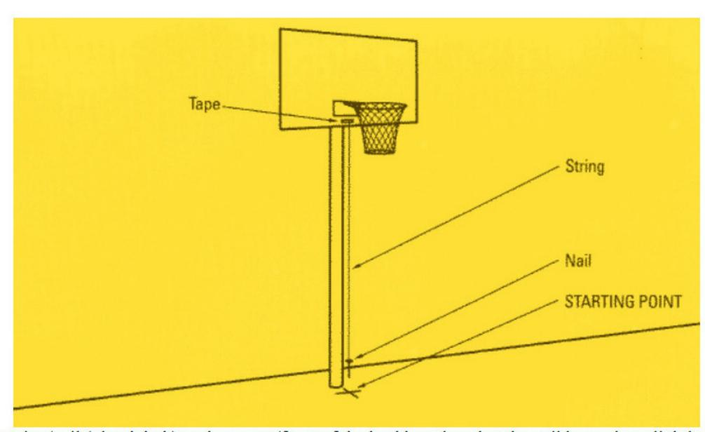
Tape the string/nail (plumb bob) to the center/front of the backboard so that the nail hangs just slightly above the court surface. The nail indicates the STARTING POINT
