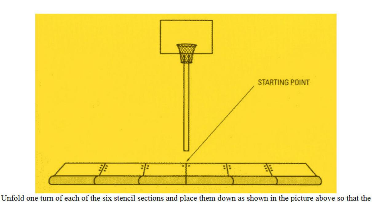
starting holes line up like dominos. The corners of the two panels with single starting holes meet at the starting point.
