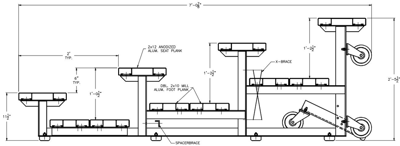
**NOTE:** ILLUSTRATION SHOWN WITH DOUBLE FOOT PLANK AND NO RISER.
