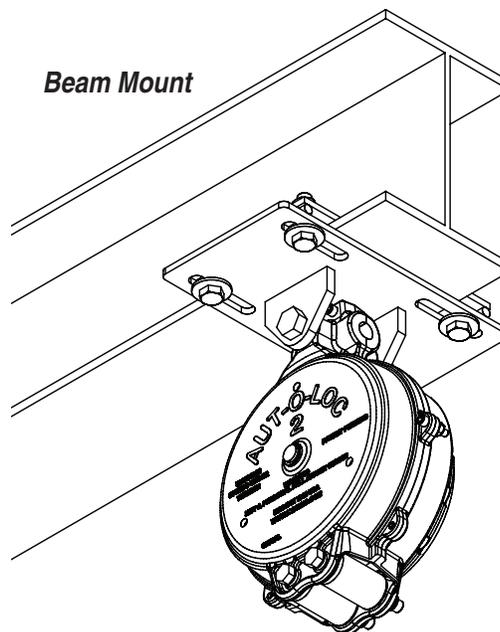
**Tube and Beam Mounts can be mounted either parallel or perpendicular to the tube or beam. Tube Mount is shown perpendicular; Beam Mount is shown parallel.**
